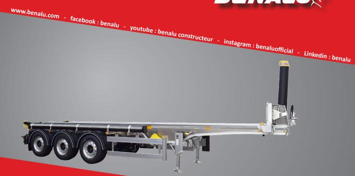
**Type: Tipping container chassis** Material: Aluminium Adaptability: 20', 30', 40' **Use: Intermodal** Approved for combined transport
